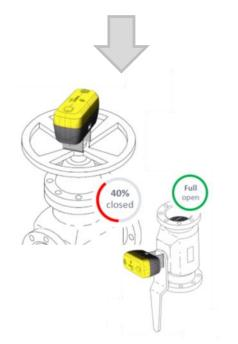
**New situation:** Manual valve positioning device measures exact position of any manual hand valve
