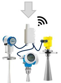
**New situation:** Industrial Tank level radar meters connect via 4-20 mA or Modbus to LoRa transceiver; no multicores required
